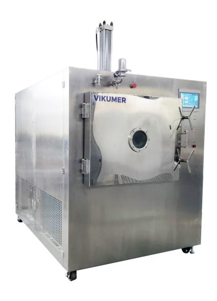
Vikumer's BFD-20 pilot freeze dryer suits small volume production in non-aseptic industries, clinical trials, process optimization and preparation of technology transfer to later commercial production.
